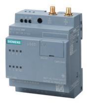
LOGO! CMR2040 communication module for connection LOGO! 8 to LTE network; 1 RJ45 port for Ind. Ethernet connection to LOGO! 8; 2xDI; 2xDO; write/read access to LOGO! variables; SMS dispatch/ receiving of text messages; email dispatch; position detection GPS; time synchronization/ forwarding with real time clock; Configuration/diagnostics via web interface; Remote access via OpenVPN/HTTPs, DynDNS, observe national approval! Manual available as a download.
